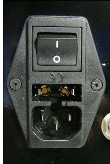
FUSE HOLDER REMOVED
